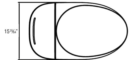
This toilet is designed to rough-in at a minimum dimension of (12") from finished wall to C/L of outlet. Supply not included with fixture and must be ordered separately.
