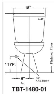
This toilet is designed to rough-in at a minimum dimension of 305mm (12") from finished wall to C/L of outlet. Supply not included with fixture and must be ordered separately.
