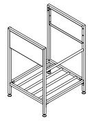
7.Screw the hand-tighten thumb screws (I) into the holes on the rack and tighten.
