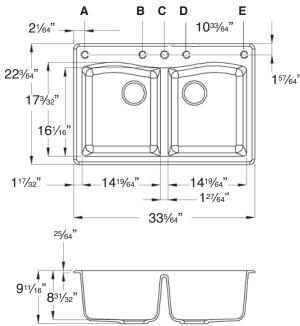
IMPORTANT: Circle Letter(s) above to indicate location(s) for faucet hole drillings (there is a 4" spread between hole locations B,C,D. There is a 1033/64" spread between hole locations A and B and D and E).
