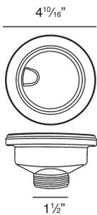
Water drains easily when cover is in place. Cover flips up with easy touch. Polypropylene housing. Fits standard 3½" opening.
