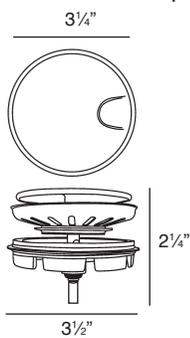
Water drains easily when cover is in place. Cover flips up with easy touch. Polypropylene housing. Top mount installation for 3½" opening.
