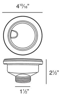
Water drains easily when cover is in place. Cover flips up with easy touch. Polypropylene housing. Fits standard 3½" opening.
