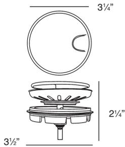
Water drains easily when cover is in place. Cover flips up with easy touch. Polypropylene housing. Top mount installation for 3½" opening.
