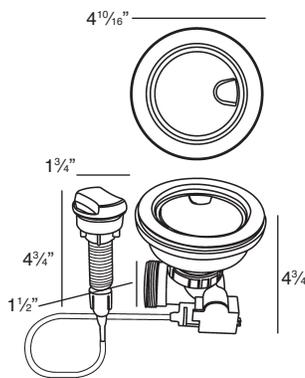
Turn the remote knob to open and close drain. Water drains easily when cover is in place. Cover flips up with easy touch. Polypropylene housing. Fits standard 3½" opening. 1 3/8" hole required in countertop for remote installation. Remote cable 25½" L.
