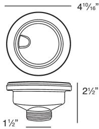
Water drains easily when cover is in place. Cover flips up with easy touch. Polypropylene housing. Fits standard 3½" opening.
