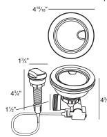
Turn the remote knob to open and close drain. Water drains easily when cover is in place. Cover flips up with easy touch. Polypropylene housing. Fits standard 3½" opening. 1¾" hole required in countertop for remote installation. Remote 4¾" cable 25½" L.
