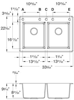
IMPORTANT: Circle Letter(s) above to indicate location(s) for faucet hole drillings (there is a 4" spread between hole locations B,C,D. There is a 1025/64" spread between hole locations A and B and D and E).
