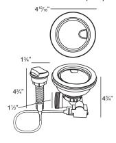
Turn the remote knob to open and close drain. Water drains easily when cover is in place. Cover flips up with easy touch. Polypropylene housing. Fits standard 3½" opening. 1%" hole required in countertop for remote installation. Remote cable 25½" L.
