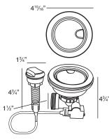
Turn the remote knob to open and close drain. Water drains easily when cover is in place. Cover flips up with easy touch. Polypropylene housing. Fits standard 3½" opening. 1%" hole required in countertop for remote installation. Remote cable 25½" L.
