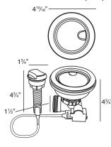
Turn the remote knob to open and close drain. Water drains easily when cover is in place. Cover flips up with easy touch. Polypropylene housing. Fits standard 3½" opening. 1%" hole required in countertop for remote installation. Remote cable 25½" L. 4010 Covered Flip Top Disposer Strainer.
