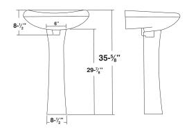
Dimensions shown for location of supplies, waste and mounting clips are suggested. Installation instructions supplied with lavatory. Mounting clips included.
