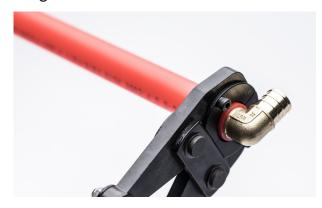
Place the fitting into the crimping tool. The crimping jaw must be perpendicular to the pipe. Then, close the jaw of the tool until it is completely closed.
