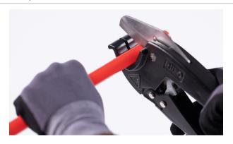
**STEP 1**Quickly and precisely cut the pipe vertically.
